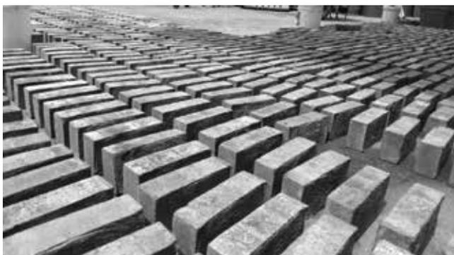
**Figure 2.** Biobrick that was built by Biomason.
